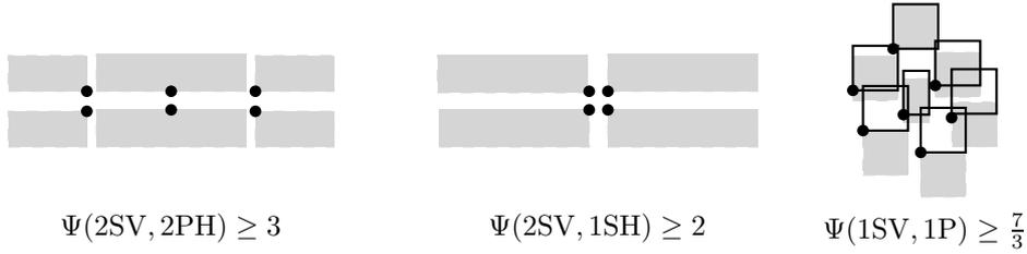
Figure 3: Lower-bound examples for one-way sliding.
