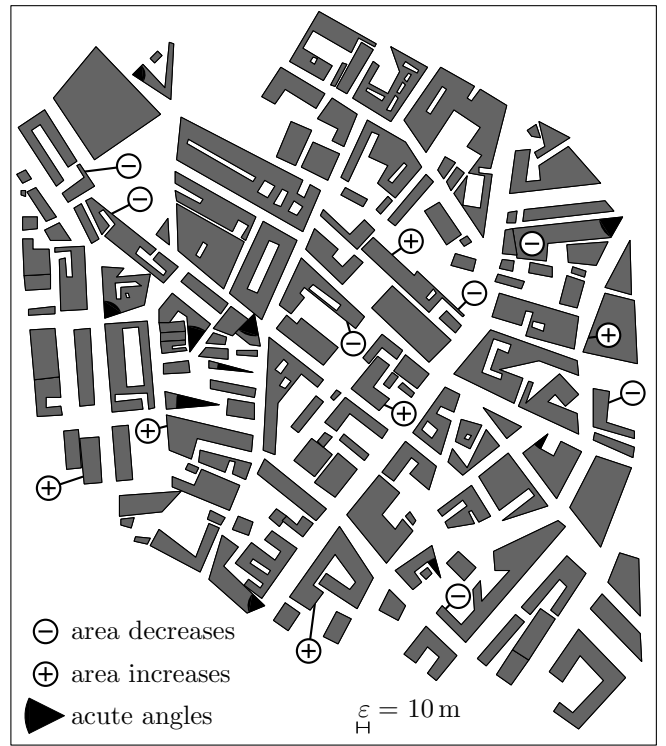
Figure 9: Result of our algorithm minimizing the number of vertices subject to the error tolerance \varepsilon = 10 m.
