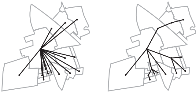
Figure 7: Measures for compactness: Based on direct distance (left) and based on adjacency graph (right).
