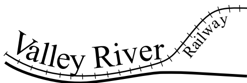
Figure 3: The label Valley River is badly placed because there is another feature between the label and the feature it labels. The label Railway is badly placed because it is below its feature.
