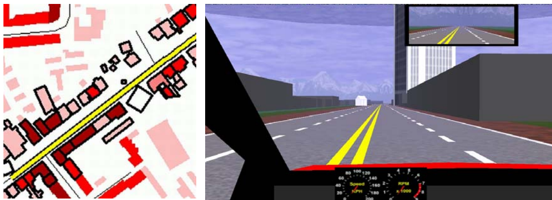
Figure 7: Example of a driving simulator scene with GIS data on the left and derived simulator scene on the right. The simulation route is shown in yellow and starts close to the lower left corner. Other roads of the road network are shown as thin black lines. Grey buildings in the scene were automatically generated from the ground plans shown in red in the GIS. The white skyscraper building was taken from the building library of STISIM and inserted manually. It appears in the GIS in white on the right hand side of the road.
