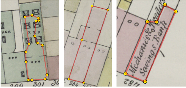
Figure 2: The polygon on the left is semantically incorrect because it does not represent a building footprint. The polygon in the middle is also incorrect, because it has one vertex too many. The polygon on the right has inaccurate vertex positions, but is semantically correct because it covers the right shape and has exactly one vertex for each corner.
