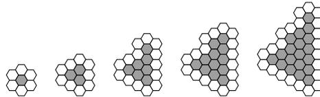
■ **Figure 7** A demonstration of the column-counting algorithm. Each polyhex is generated by one iteration of the algorithm.
