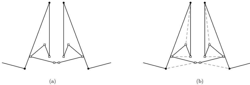
■ **Figure 1** (a) This gadget allows for simulating a “bend” in the polygon without a vertex that needs to be matched. The construction is scaled such that the eight points marked with squares do not see any other point outside of the gadget (in particular, narrowing it horizontally). (b) A possible matching is shown.
