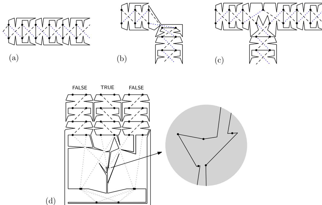
■ **Figure 2** (a) A wire gadget and its two truth states (one in dashed, the other in dotted). (b) A bend in a wire gadget. (c) A split gadget that transports the truth setting of one wire to two other ones. This is used for representing the variables. (d) A clause gadget. The visibility among the vertices of degree two is indicated by the lighter lines. Exactly one vertex of degree two of the part in the circle must be connected to a wire above that carries the true state.
