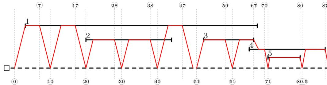
■ **Figure 3** Scenario with 5 scenes represented by solid black lines. The dashed black line represents the base. The red solid stroke represents the movement of the drone following an optimal solution. The battery lasts 10 units of time. Closed in gray circles are the time instants associated to the drone's moves.
