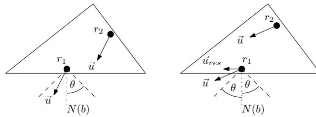
■ **Figure 2** Left: An input force command  $u(t)$  within the cone  $\pm\theta$  about the normal to the boundary results in no motion of  $r_1$ . Right: An input force command  $u(t)$  outside the cone results in a motion of both particles. Observe that  $r_1$  slides along the boundary with a resulting force  $u_{res}(t)$ .
