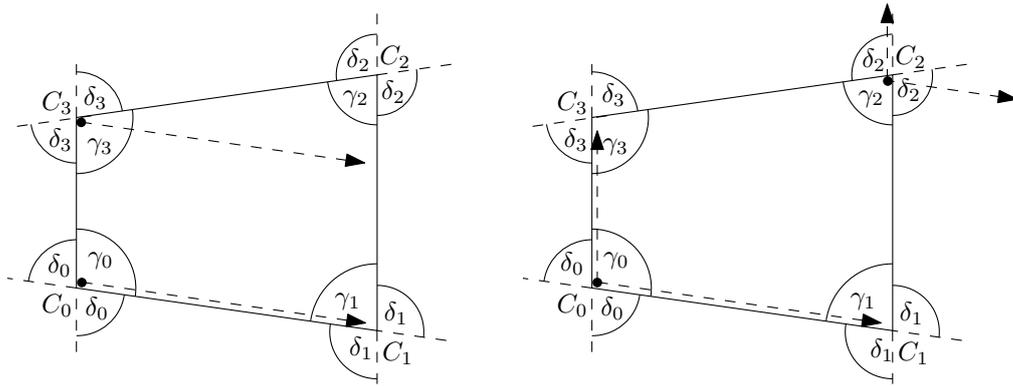
Figure 6 Left: Particle in  $C_0$  cannot be moved without moving a particle in  $C_3$ , because  $\delta_0 < \gamma_3$ . Right: However, we can move the particle in  $C_0$  to any place in the polygon without moving a particle in  $C_2$  (unless the friction is too small), because  $\delta_3 + \delta_0 > \gamma_2$  and  $\delta_1 + \delta_0 > \gamma_2$ .
