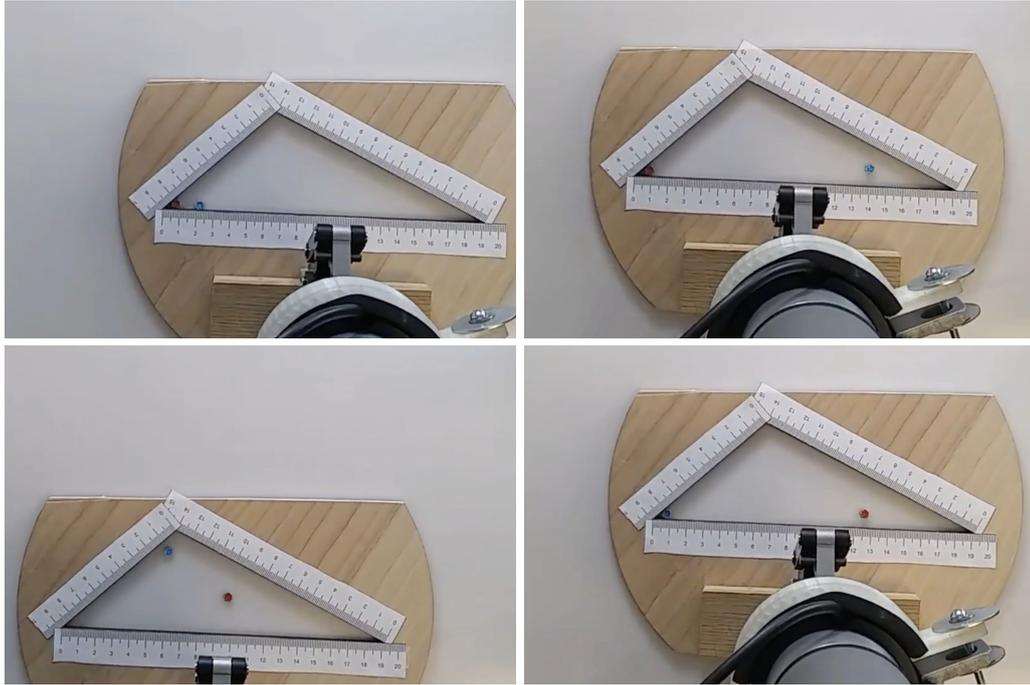
■ **Figure 1** A robot arm moving a triangle to reconfigure two particles. Top left: Two particles are close together. Top right: Blue particles has been separated from the red particle with zig-zag moves. Bottom left: Situation after a south-east and a south-west move. Bottom right: After the blue particle is kept in the bottom left corner, the red particles is moved away with zig-zag moves.
