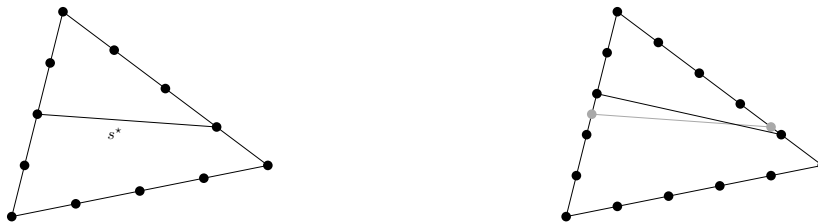
Fig. 6.3: Three Steiner points evenly distributed along the triangle edges achieve the optimal path segment. By increasing m to 4, all Steiner points shift on all edges and the optimal segment cannot be found anymore. This results in worse approximation with a bigger value for m .
