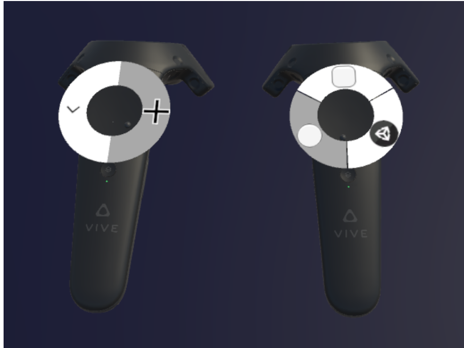
Figure 3.2. Menus attached to the controllers. Each menu item can be used by pressing the touchpad in the corresponding sector of the circle
