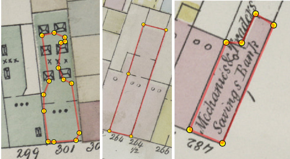
Fig. 6.2: The instance on the left is semantically incorrect because the polygon is certainly not representing a building. The image in the middle is also not correct because it has one corner too many. Even if there are two inaccurate points on the right picture, this polygon is semantically right because it covers the correct shape and has the proper amount of corners.
