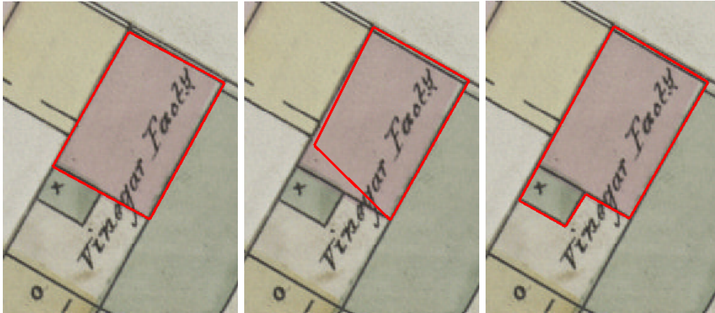
Fig. 6.3: The leftmost polygon is correct and has an average brightness of 0.36, the polygon in the center has an average brightness of 0.48, but it is semantically correct. The last polygon has an average brightness of 0.38, which is pretty small. However, the polygon itself is not useful.
