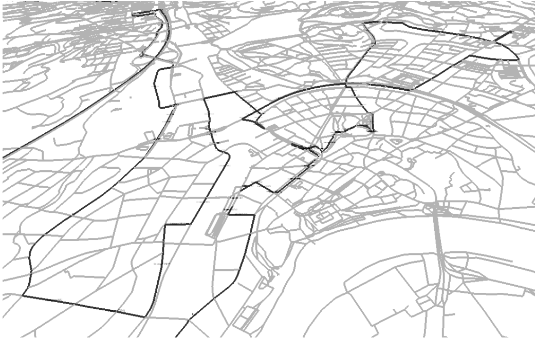
Figure 2: Bird's eye view of a plotted route through the street network in Lower Franconia. The seemingly random route was calculated using a depth-first-search algorithm with road data from OpenStreetMap.
