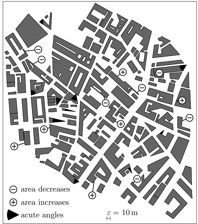
Figure 9: Result of our algorithm minimizing the number of vertices subject to the error tolerance \epsilon = 10 m.
