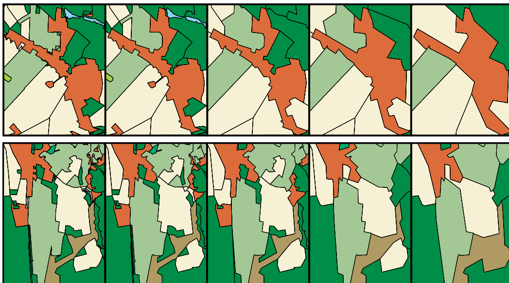
Fig. 5. Two examples processed with Algorithm 1. From left to right: Original map, found intermediate representations, and map generalised by optimisation.
