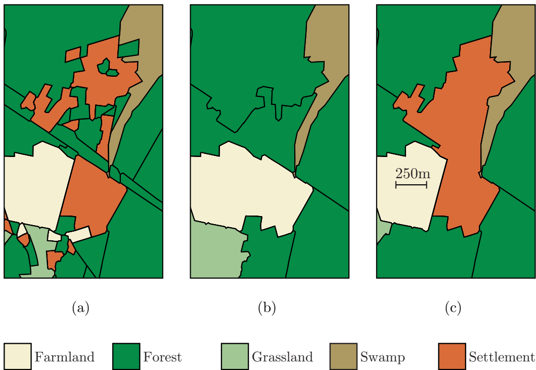
Fig. 1. Comparison of two aggregation methods: (a) Input data set ATKIS DLM50, (b) result of iterative merging, (c) result by optimisation; both results satisfy size constraints defined for the ATKIS DLM250.
