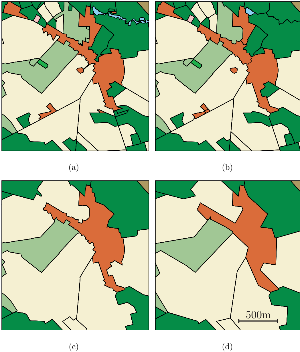
Fig. 3. Applied generalisation steps: (a) original map , (b) after collapse by skeletons, (c) after aggregation, (d) after line simplification.
