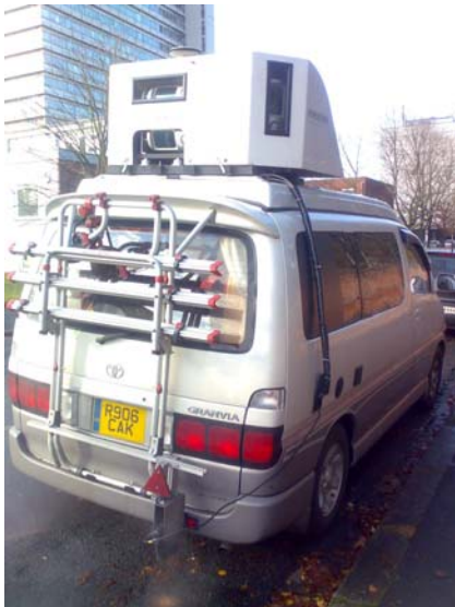
Figure 8: The streetmapper system used to acquire the scan in which point features (poles) were detected. The system comprises four terrestrial laser scanners, a GPS antenna (on top of the van), an odometer (mounted close to the bumper), an IMU, and a control computer.
